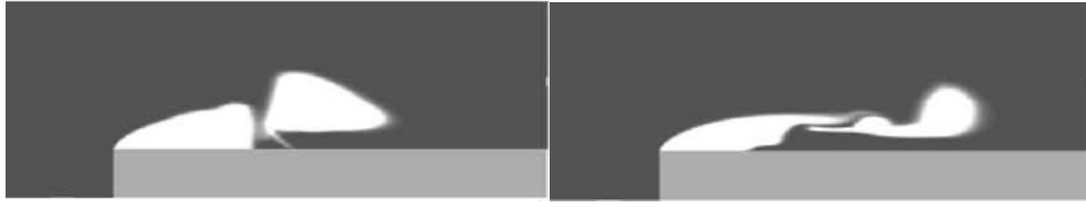
Figure 6-10: Cavitation evolution by Zhang et al. [76]. Attached cavitation shown in white.
