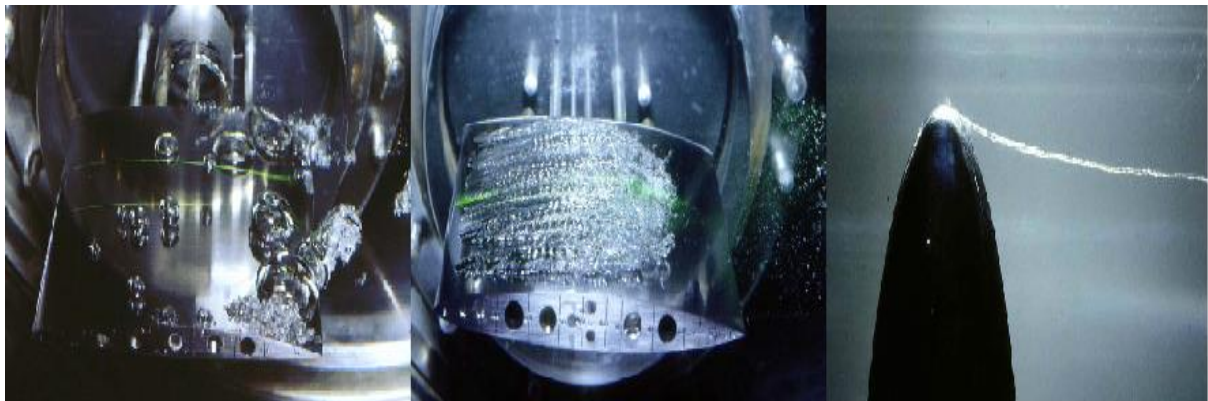
Figure 4-10: Travelling, attached and vortex cavitation (left to right). Figure based on Franc [59].
