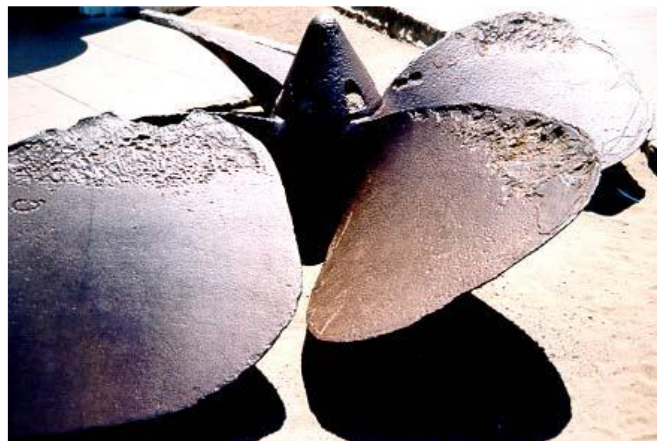
Figure 4-18: Material erosion on ship propellers caused by vortex cavitation collapse. Figure reproduced from Senocak [73].
