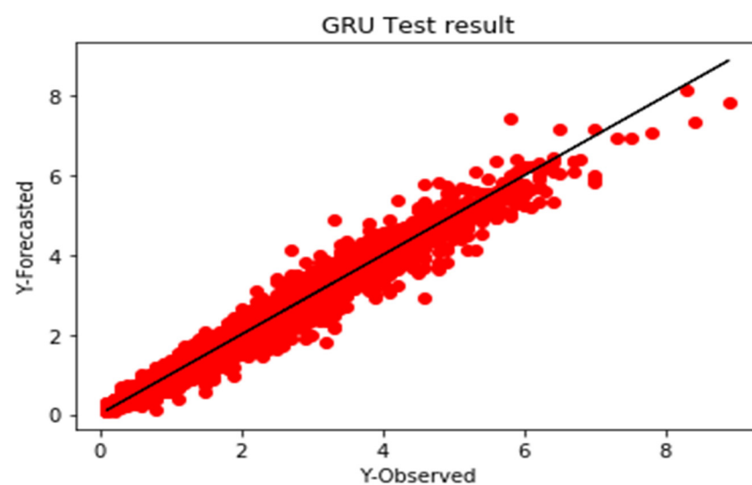
Figure 22. GRU-based wave height model error analysis.
