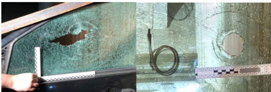
Fig. 6 Fracture pattern post impact by a 2219 bolt and EK Bolt in to window 1 and 6, respectively
