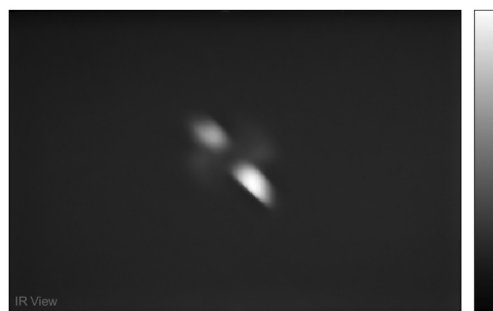
(e) 20J impacted thick specimen
