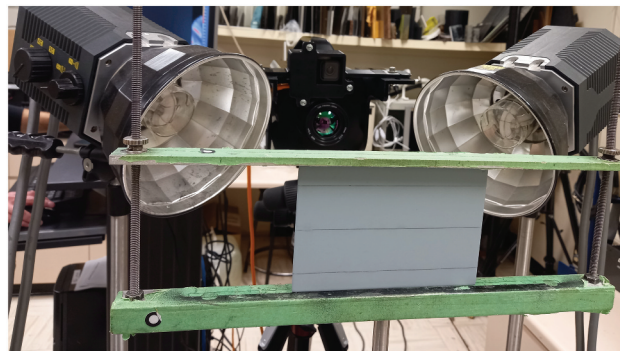
Figure 1. PT experimental setup in reflection mode with a BVID specimen.
