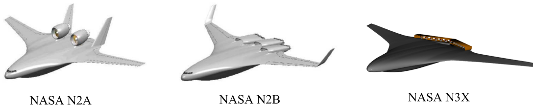
FIGURE 2.3: Summary of the main BWB configurations for different levels of propulsion integration. N2A and N2B from Kim et al. 7 , N3X adapted from the sample OpenVSP hangar configuration 8
