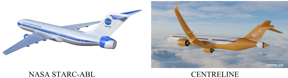
FIGURE 2.7: Aft-mounted annular propulsor configurations. STARC ABL configuration from Gray et al 11 . CENTERLINE concept from Seitz et al 12
