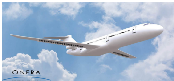
FIGURE 2.4: Wing mounted distribution propulsion concept by ONERA: DRAGON (Distributed fans Research Aircraft with electric Generators by ONERA)from Schmollgruber et al 4
