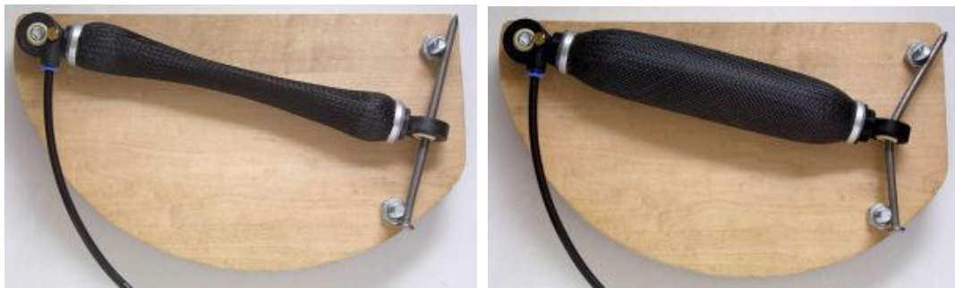
Figure 2-15 Air muscle extension and extraction
