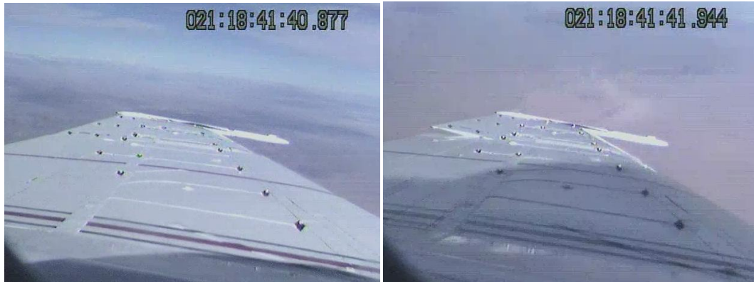
Figure 2-8 Test video captured F/A-18 AAW aircraft control surface motion while rolling
