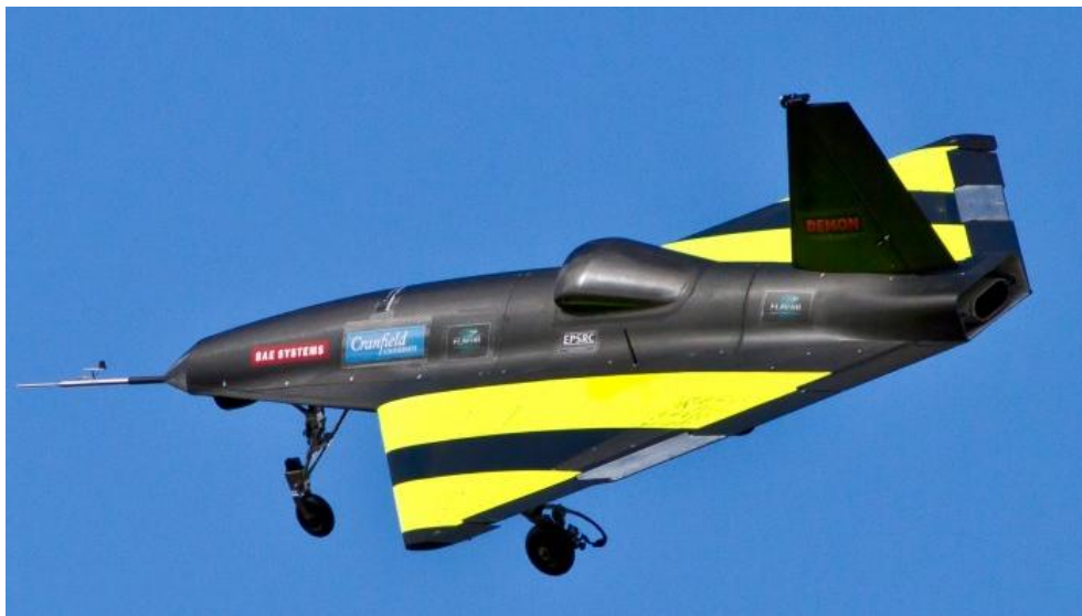
Figure 1-2 Flapless flight demonstration UAV “Demon”
