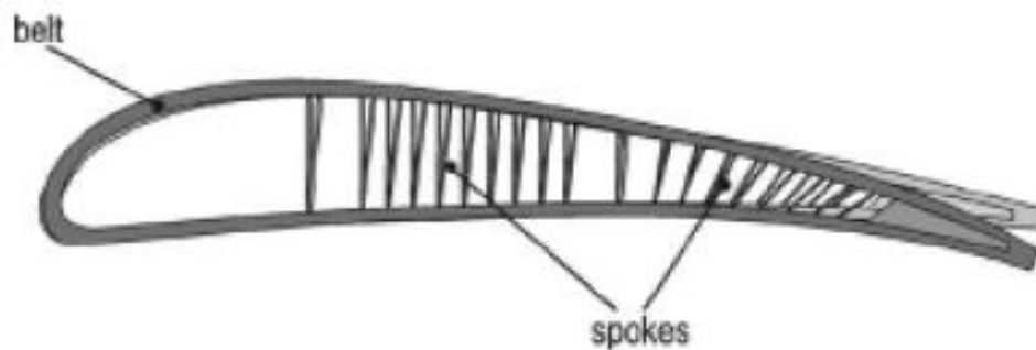
Figure 2-11 Belt-rib morphing concept
