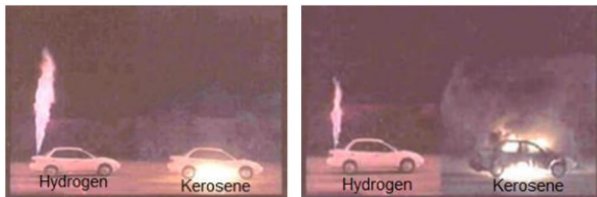
Figure 2-36: Safety comparison between a Hydrogen and Kerosene fuel leak [54]
