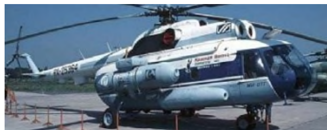
Figure 2-29: Mil-8TG helicopter operating on Propane/Butane mixtures [51]
