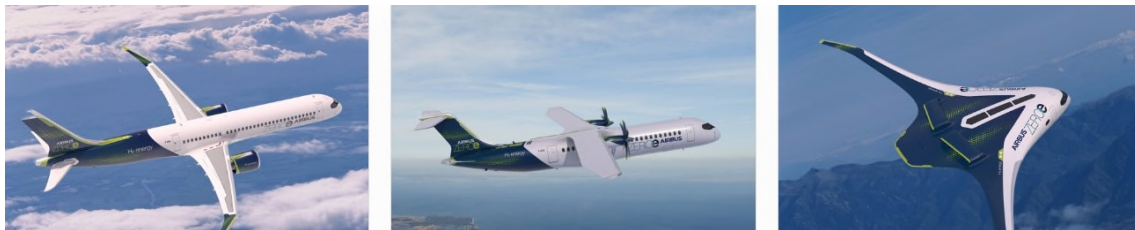
Figure 1-3: AIRBUS ZEROe concepts using liquid Hydrogen [7]
