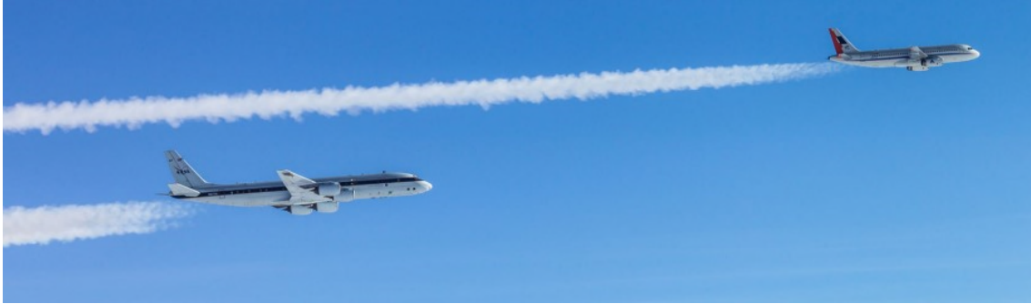
Figure 2-12: The NASA DC8 research aircraft probing contrails from the DLR A320 burning sustainable aviation fuel blends [41]
