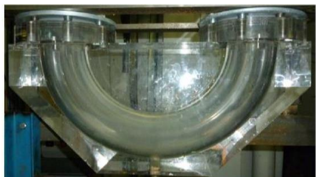
(c) Close up of return BEND2
