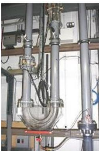
(b) Bottom section showing return BEND2, viewing section, and instrumentation
