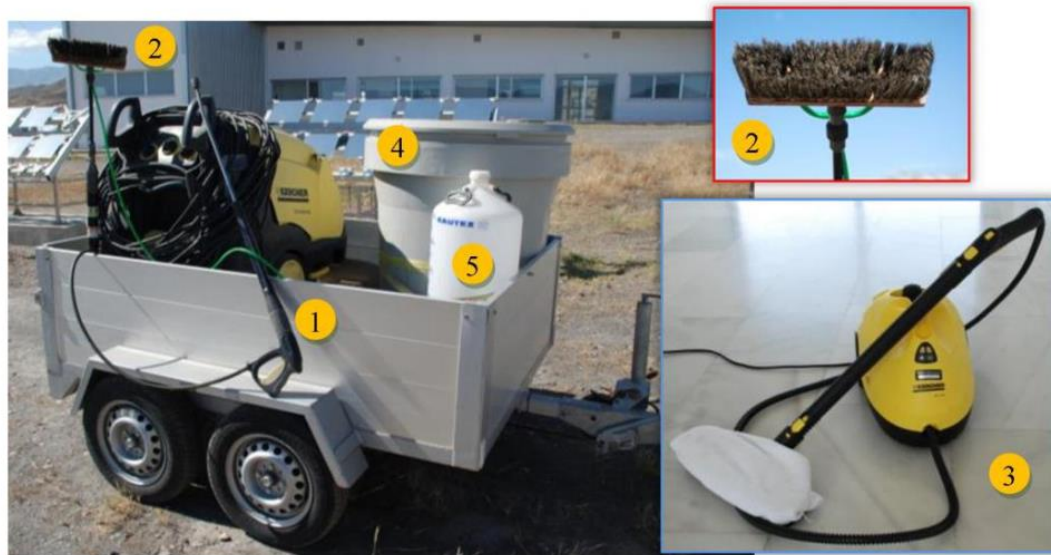
Figure 2-16 Typical equipment for manual cleaning of mirrors. Items are labelled by: 1: pressure washer with handheld nozzle, 2: water-fed horsehair bristle brush attachment, 3: steam cleaner, 4: demineralised water tank, 5: detergent tank [3].
