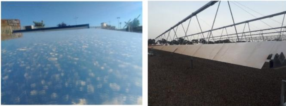
Figure 2-15 Photographs showing soiling of mirrors at IMDEA Energy, Spain (Left), and Green Energy Park, Morocco (Right) [46].
