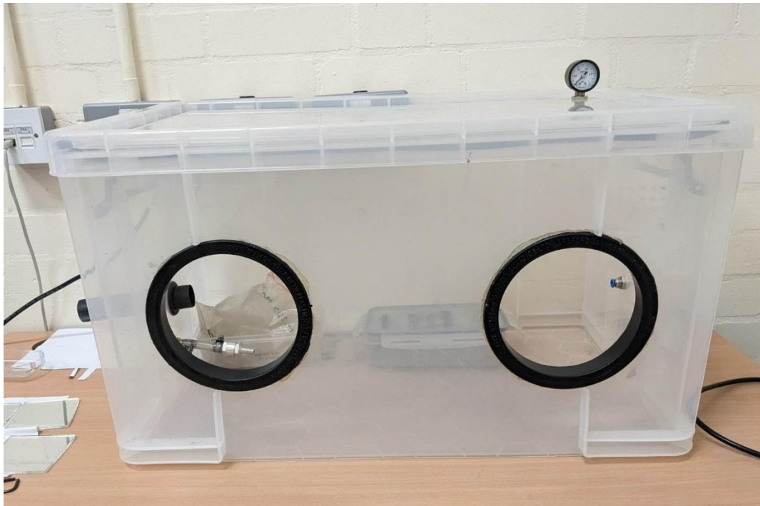
Figure 5-6 Photograph of soiling chamber.
