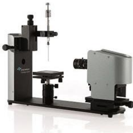
Figure 5-2 Stock photograph of a Theta Lite optical tensiometer of the same model used in this work [193].
