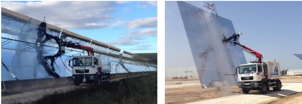
Figure 2-17 Conventional semi-autonomous cleaning of parabolic trough (left) and flat heliostat (right) mirrors [55].
