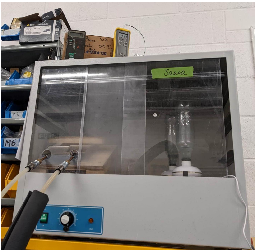
Figure 5-14 Photograph of condensation chamber.
