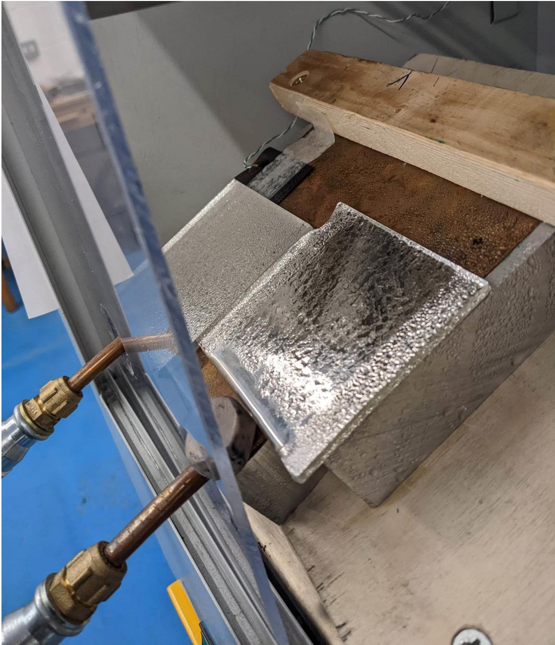
Figure 5-15 Photograph of two mirror samples on the condensation block.
