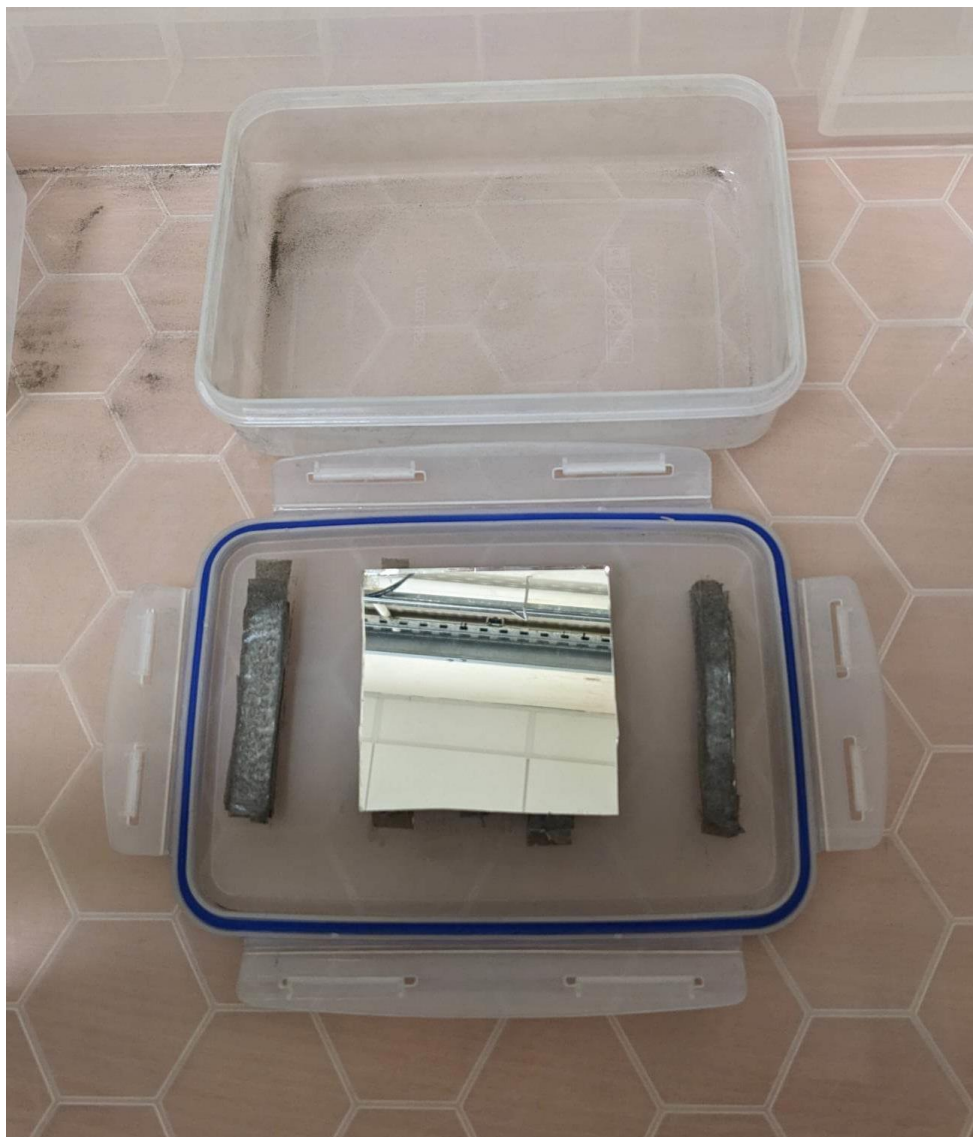
Figure 5-7 Photograph of sample mounted inside inner soiling box.
