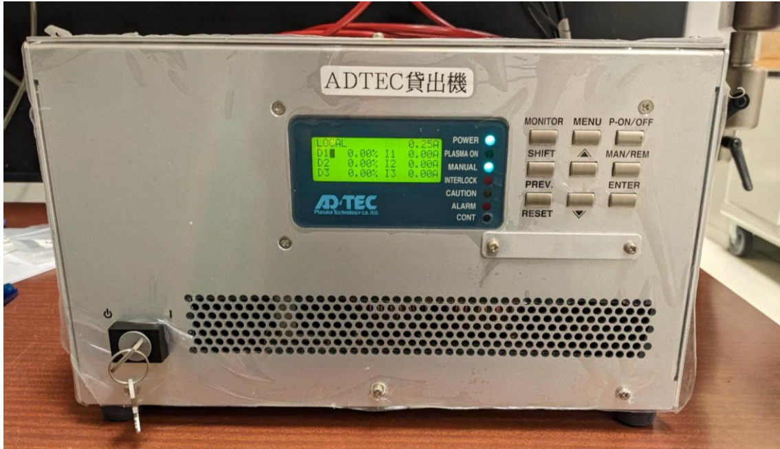
Figure 3-7 Photograph of generator used for the M-CCMD torches.
