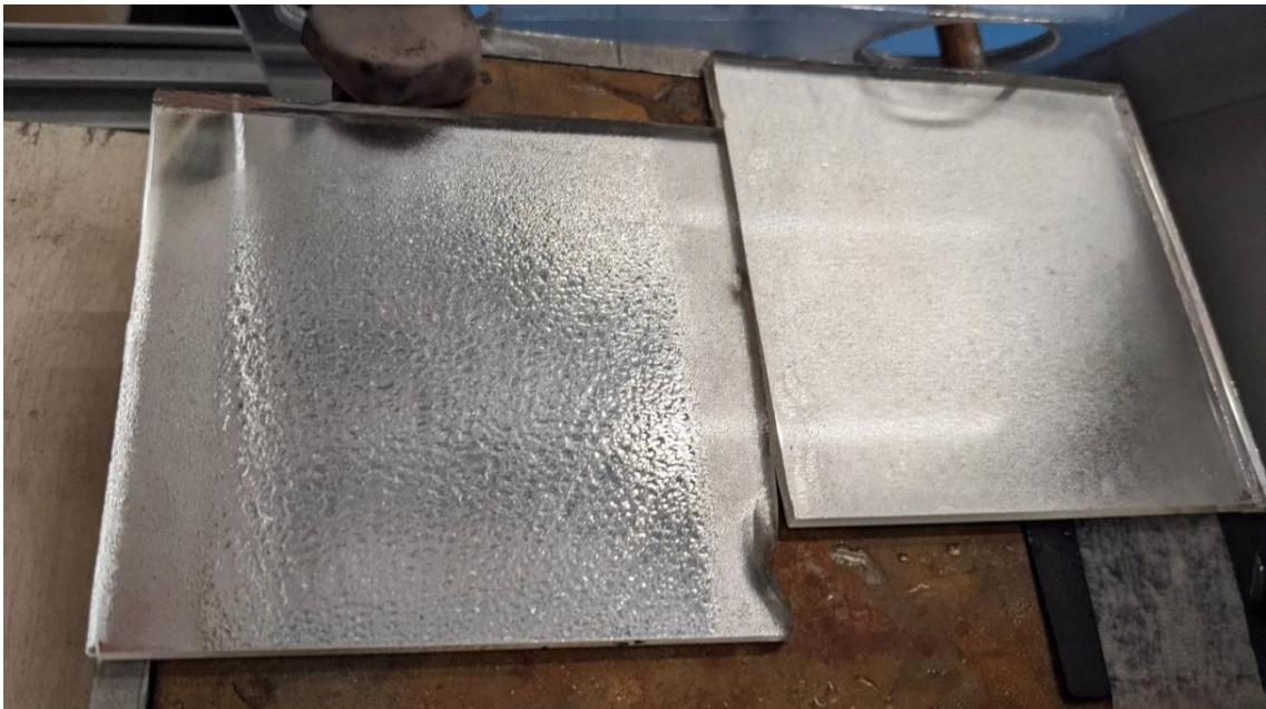
Figure 10-2 Mirror samples that have (left) and have not (right) been plasma processed, after being in the condensation chamber for 30 minutes.
