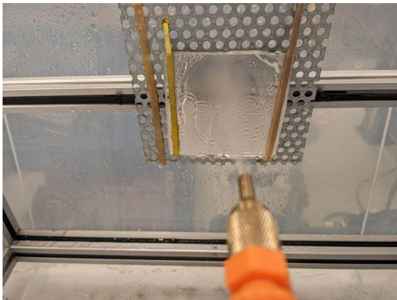
Figure 5-12 Detail of a mirror sample passing through the washing jet.
