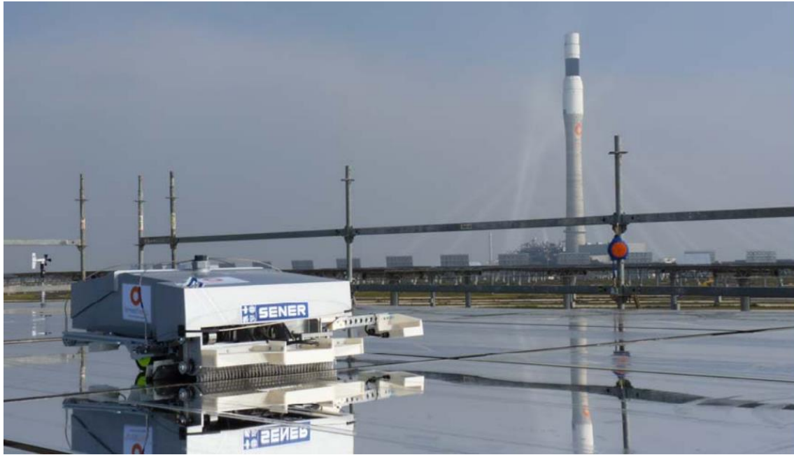
Figure 2-18 Photograph of HECTOR robot undertaking heliostat cleaning at the Gemasolar solar plant in Andalusia, Spain [58].
