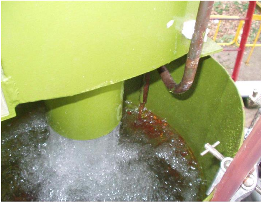
Figure 1-3 BS EN 1825 test apparatus – light fuel oil introduction to water flow (Forty 2005)
