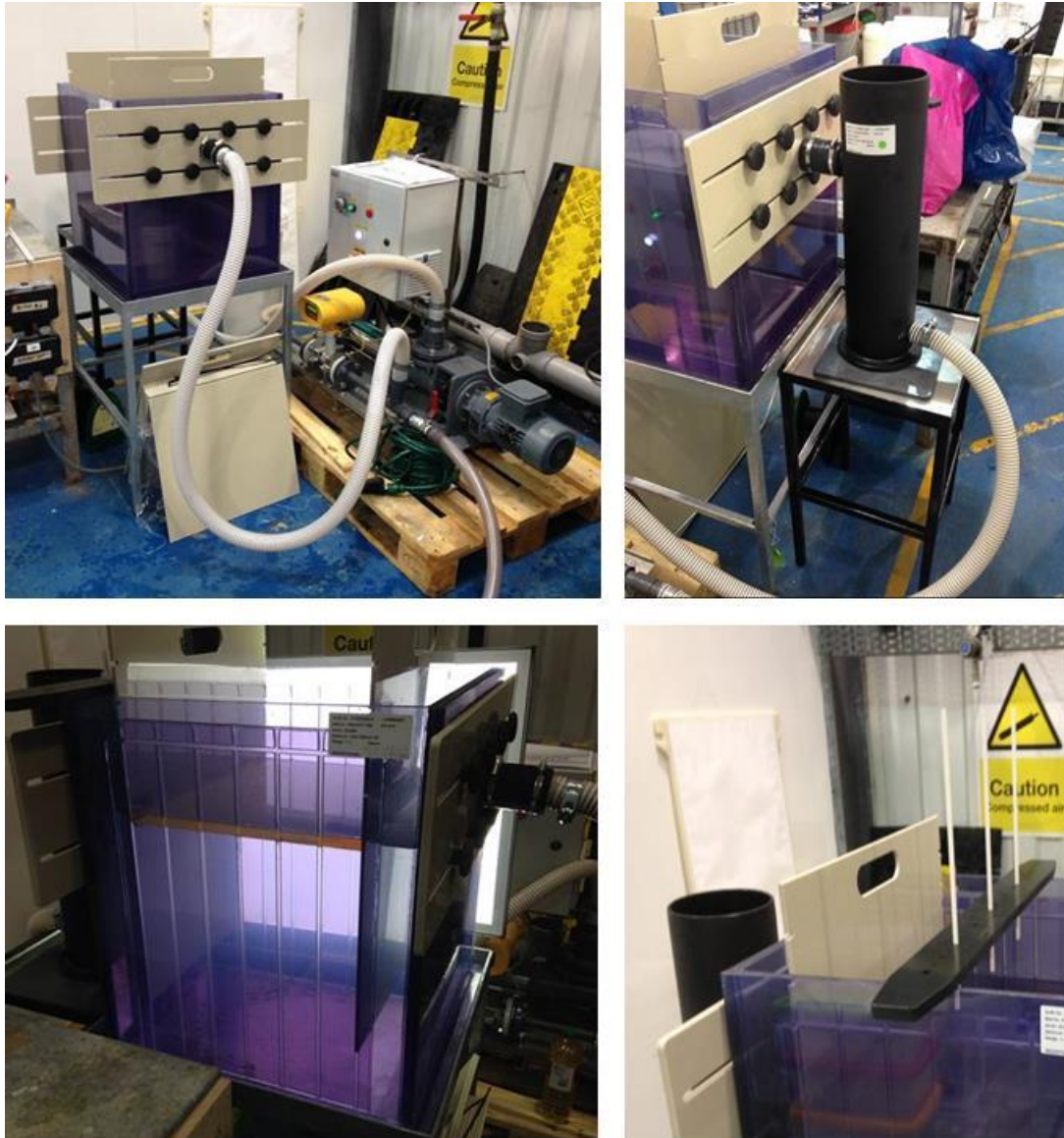
Figure 5-2 Images of apparatus. Top left - apparatus showing separator, connecting pipework, pump, flow meter, and flow control. Top right – oil water reservoir / injection point. Bottom left - transparent separator illuminated by LED with oil layer in oil separation zone. Bottom right – sampling apparatus support and 3mm PE pipe (sampling position would be to the left of the baffle plate)
