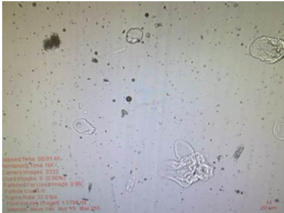
Figure A2-1 Candidate FOG droplet near centre and lighter near transparent food debris.
