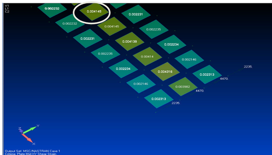
Figure 5-26 – Level 2, N_{xy} Load Case: Element 25 highlighted by a white circle
