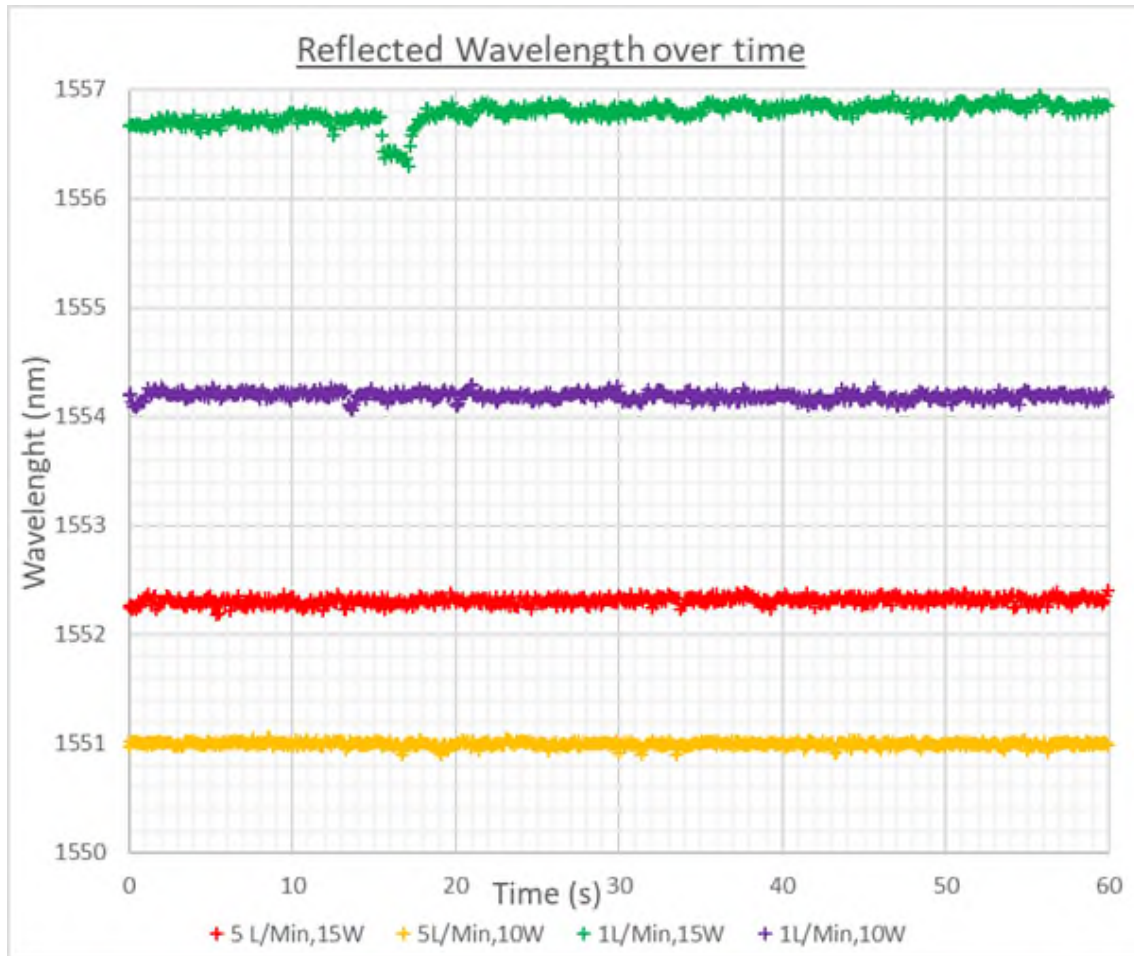
Figure 31 Reflected wavelength measurements of a static FBGS over 1 minute. Results show lower flow rates produced higher temperature readings.
