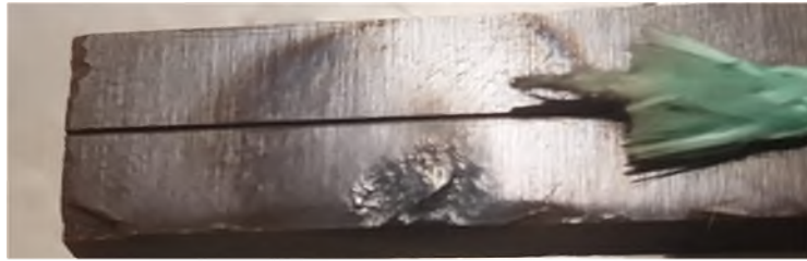
Figure 6 displaying the effect of cool microwave plasma at 15W and 5Lmin flow rate on Tufnol.
