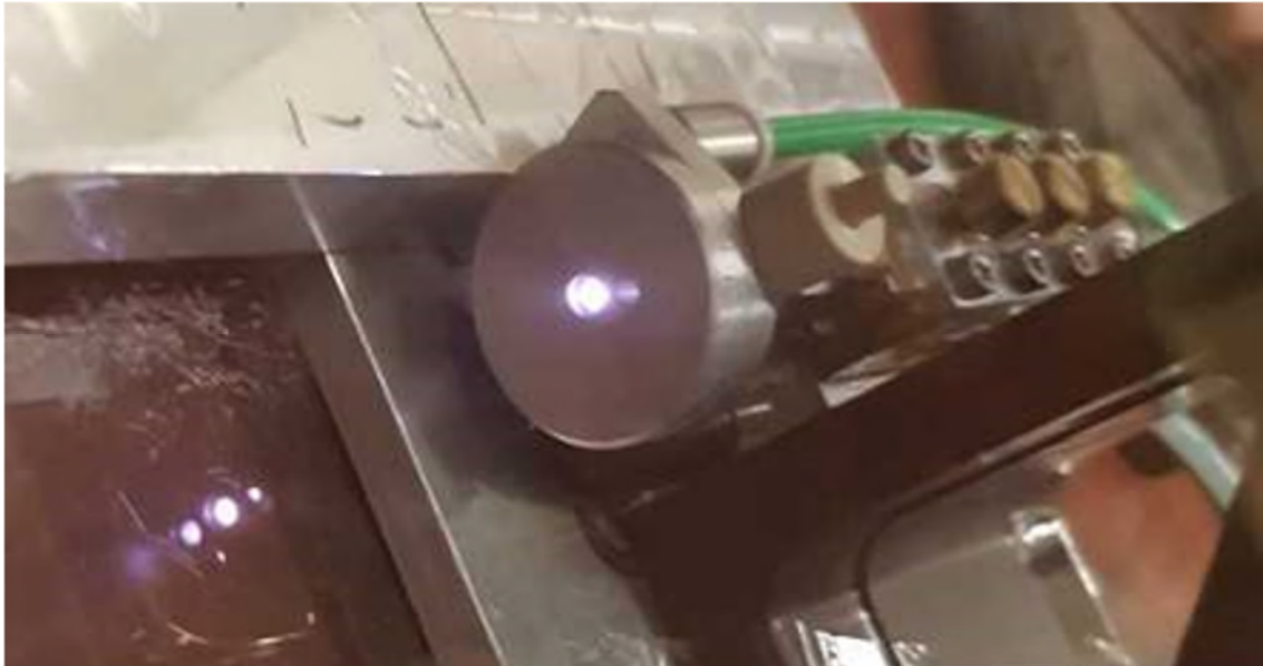
Figure 14 displaying the Plasma tact emitting a non-thermal microwave plasma jet
