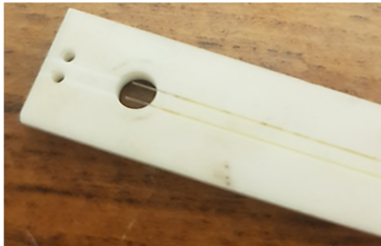
Figure 8 displays the MACOR substrate with two FBGS attached. Two 0.3mm wide grooves were milled into the substrate at a depth of 0.25mm.
