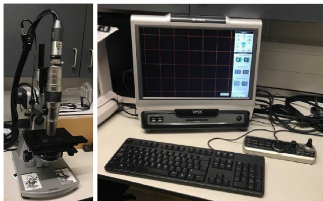
Fig. 6. High magnification VHX series digital optical microscopy.
