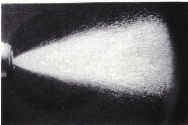
(c), P_{\text{air}} = 3 ats., Main dribbling
