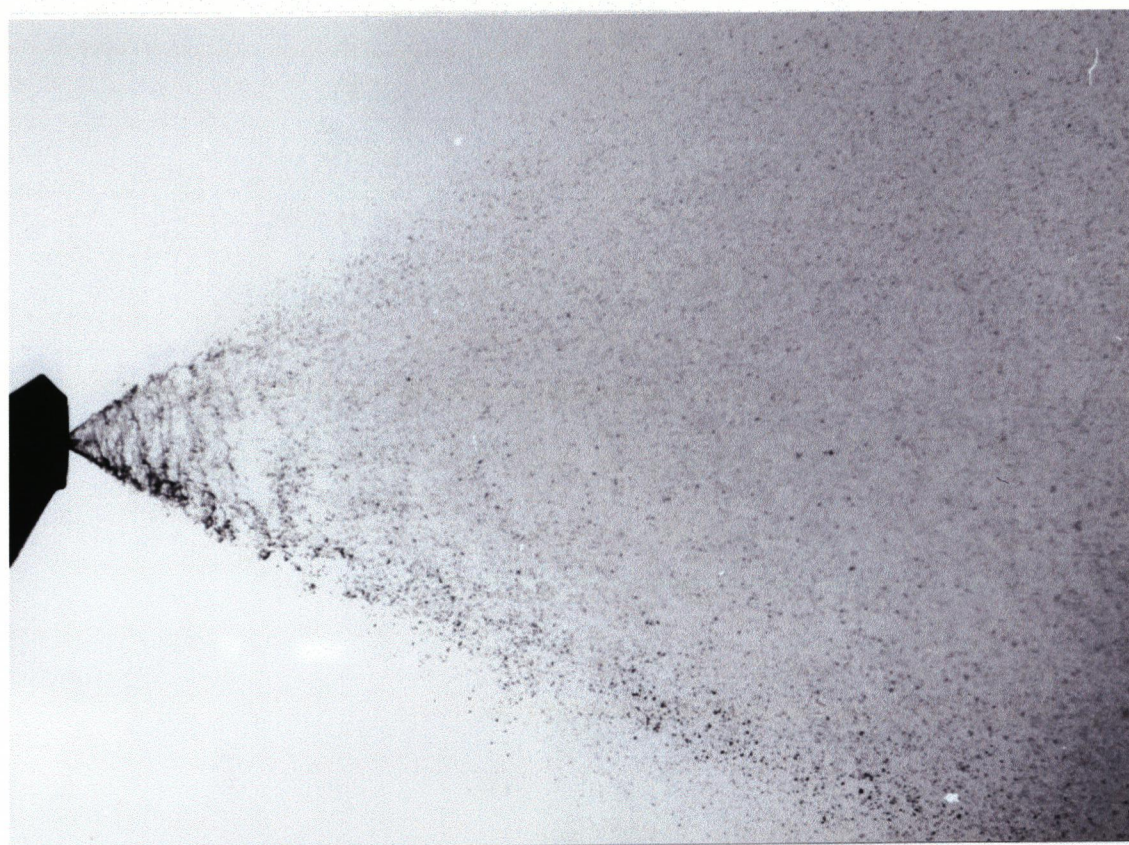
(b) High Speed Spark Photography
