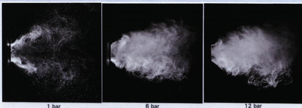
Fig. 3 Influence of air pressure on spray structure for a constant fuel flow; m_F = 5 \text{ g/s}
