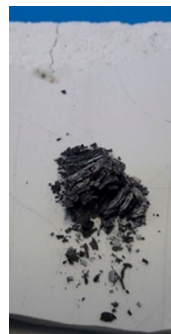
Figure 2. Mg-silicide uncoated after aging at 500 °C for 120 h, in air.
