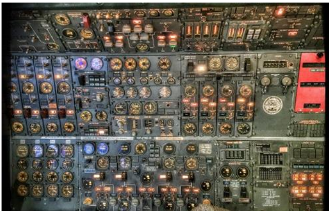
Figure 1: Part of the flight engineer control panel. Many of these systems have been now automated leading to the removal of this role in all modern civil aircraft.
