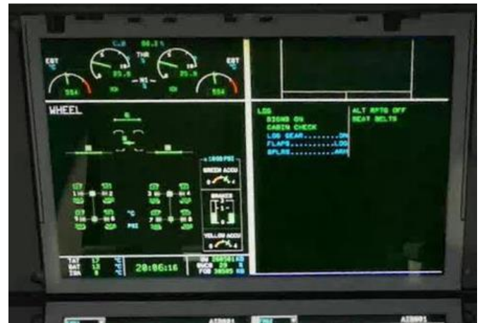
Figure 2: Modern engine indications. The presentation has changed from Figure 1 but in essence, the parameters shown have their roots in the flight engineer panel.
