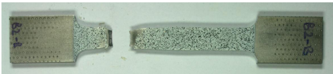
Figure 3-10: Painted tensile specimen after DIC testing
