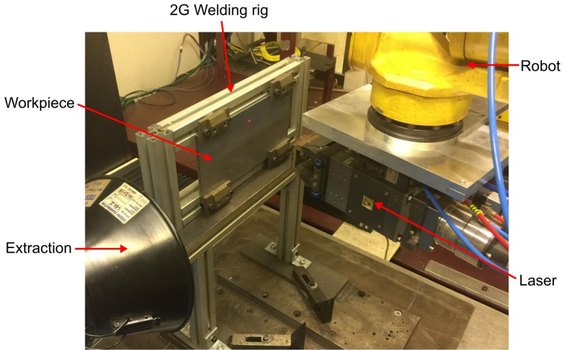
Figure 3-1: Experimental set-up for autogenous laser welding
