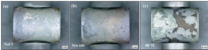
Fig. 9 Optical microscope images of the C-ring's top surface for a NaCl, b sea salt and c 80/20 mol % \text{Na}_2\text{SO}_4/\text{K}_2\text{SO}_4 after 100 h of exposure at 700 °C
