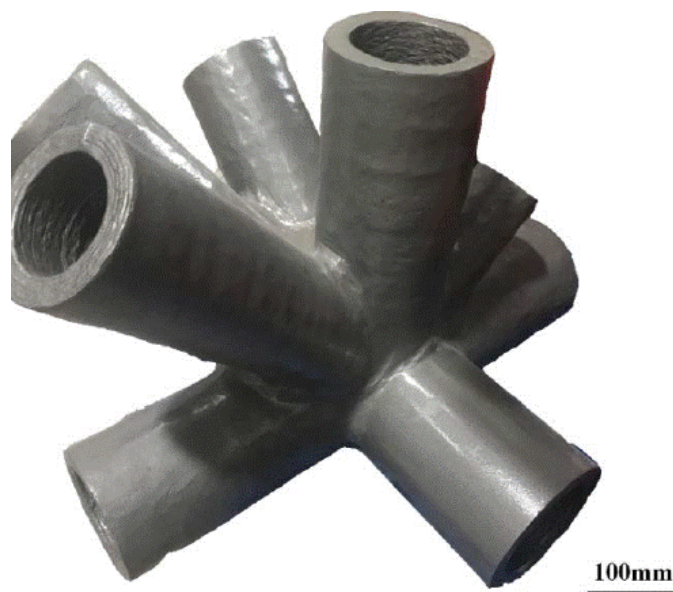
Figure 2-11 High built multidirectional HSLA steel WAA structure[38]
