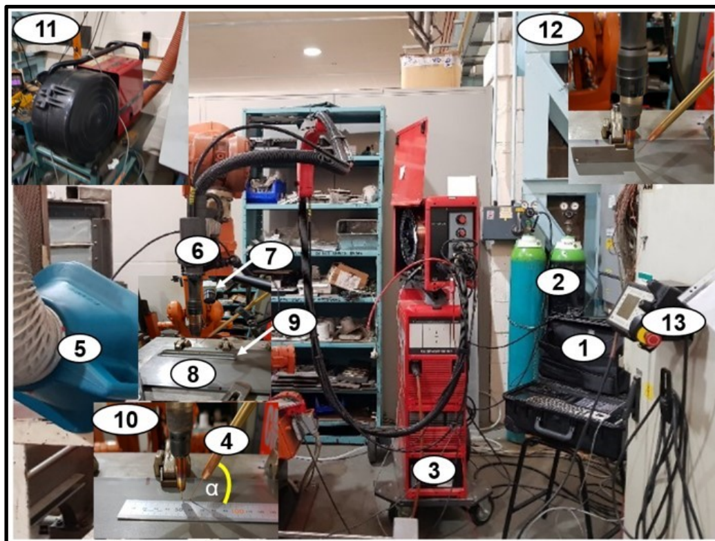
Figure 3-3 Wire assisted arc additive manufacture
