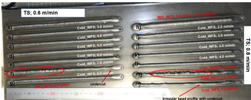
Figure 8-13 Bead profile of WAAAM (PGMA WFS at a constant rate of 8.0m/min) (a-g), TS: 0.6m/min, (h-n), TS: 0.8m/min
