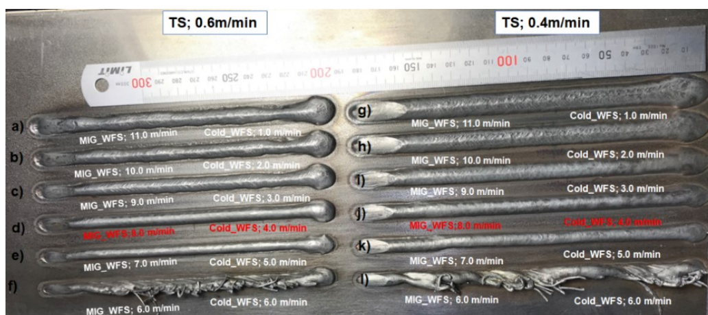
Figure 8-14 Bead profile of WAAAM (constant deposition rate of 6.27Kg/hr) (a-f), TS: 0.6m/min, (g-l), TS: 0.4m/min
