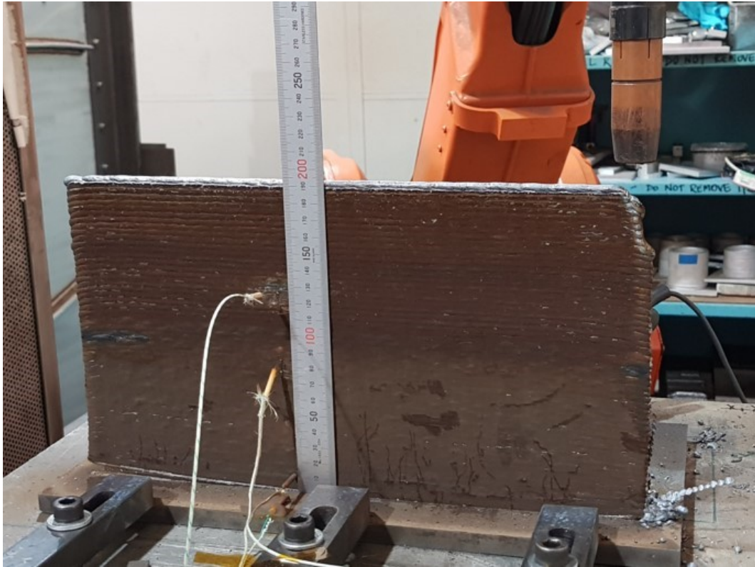
Figure 7 – WAAM built wall
