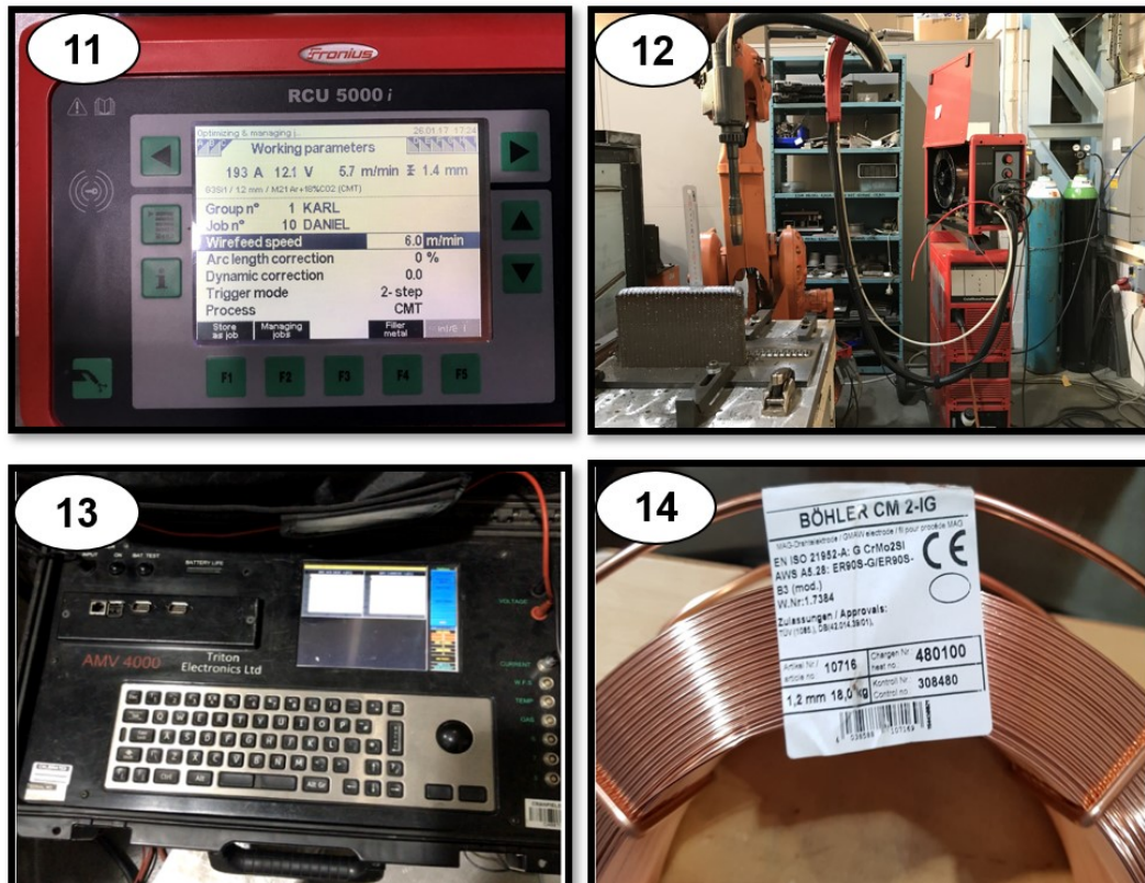
(1) ABB robot, (2) Torch, (3) CMT wire feeder, (4) Spec shield heavy, (5) Spec shield light, (6) CMT power Advance power source, (7) Clamps platform, (8) Oscillated Walls, (9) S275JR substrate, (10) Aluminium platform, (11) Fronius controller, (12) Oscillated wall, (13) AMV 4000 parameter monitor (14) Wire spool
