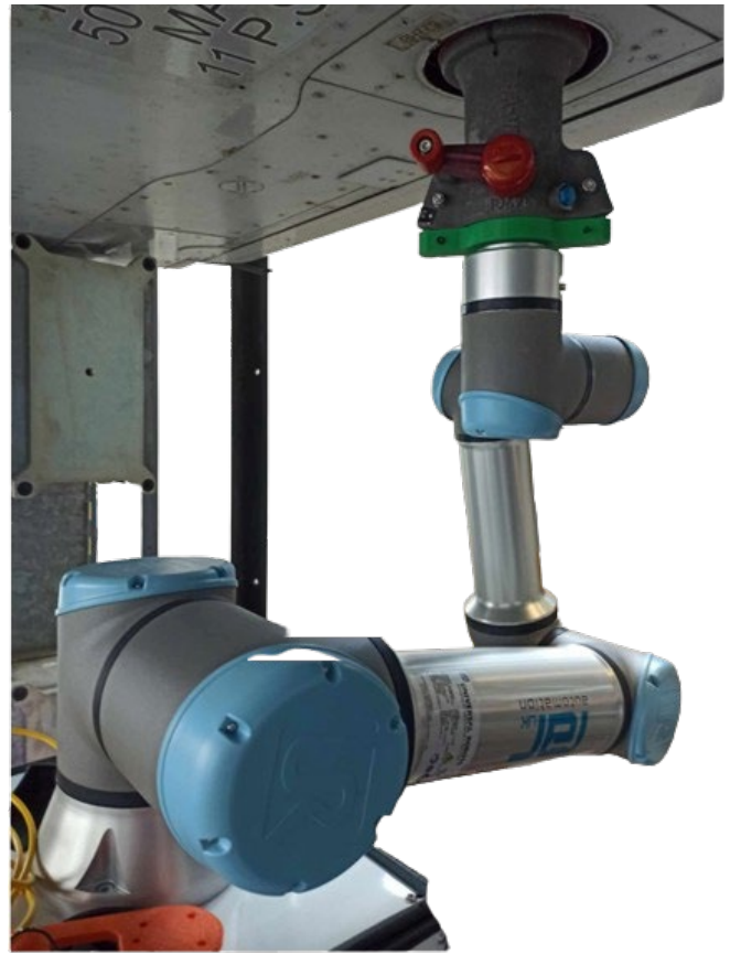
Fig.2. Initial system design using a UR16e robot with nozzle attached.
