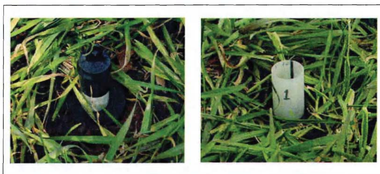
Figure 3-9 Example of a Delta-T soil moisture Access Tube installed in Church Meadow showing the rubber cap and collar fitted in an attempt to prevent water entering the tube and bypass flow down the length of the tube.
