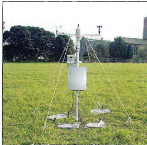
Figure 3-5 Delta-T weather station with wind vane, anemometer, net-radiometer, global radiation sensor, rain gauge, air temperature and relative humidity sensors
