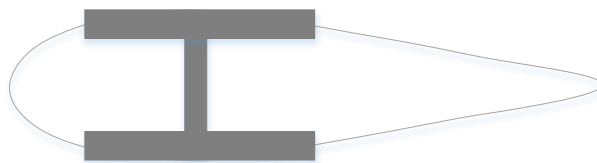
Figure 12 I beam model for bending mass calculation.
