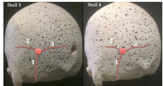
Figure 2: Crack propagation on Skull 3 and Skull 4
