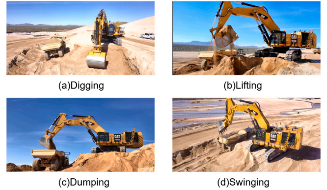
Fig. 2. The four investigated working stages/activities involved an excavator. The involvement of dumper is not essential.
