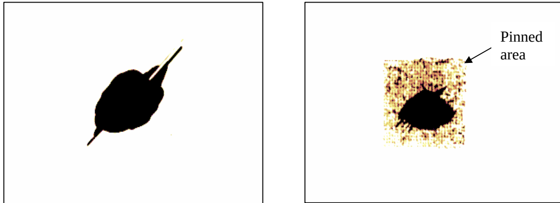
Fig. 2 C-scan images for (a) unpinned and (b) pinned 4 mm thick plates; both were impacted by 15J energy.
