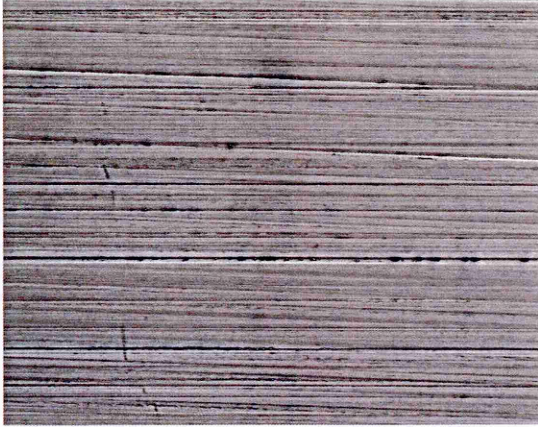
Figure 4.119: SEM from turned surface which has been electrofinished for 6 seconds + 0.2 honing only.
