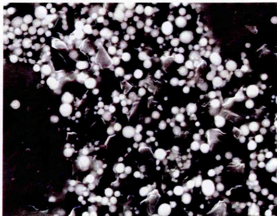
Figure 4.90a: Iron resin bonded stone (white Fe powder)
