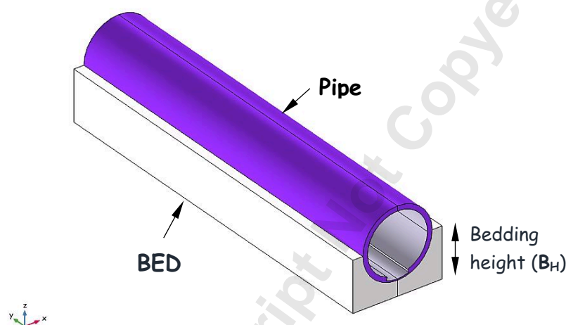
Figure 12. Description of protective bed for internally corroded pipeline
