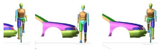
Figure 5. Cyclist and pedestrian leg positioning with respect to Large Family Car front.
