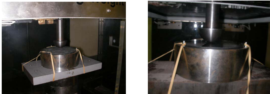
Figure 135: Punched impacted discs in the drop tower apparatus
