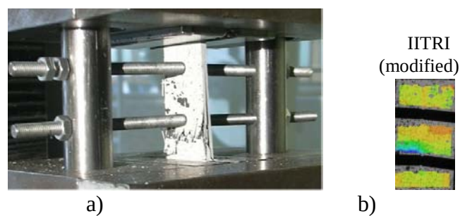
Figure 54: Failure and loading of the composite specimen in compression
