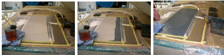
Figure 35: Resin infusion of the textile laminate
