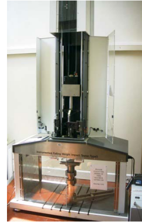
Figure 41: Drop tower apparatus
