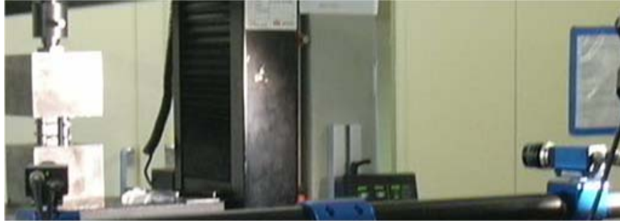
Figure 53: Strain field recording on the IITRI modified rig
