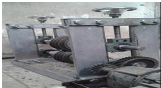
Fig. 9. Full machine frame
