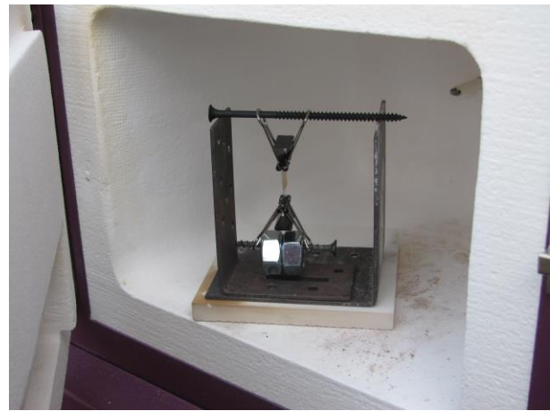
Fig. 15: Thermomechanical Demise Test Set-Up
