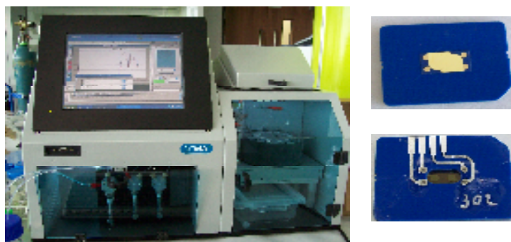
Figure 5.1: Fully automated QCMA-1 system (left) used for Salmonella detection and QCM gold sensor chip (right) with two sensing array (Sierra Sensors GmbH, Hamburg HRB 98765, Germany).
