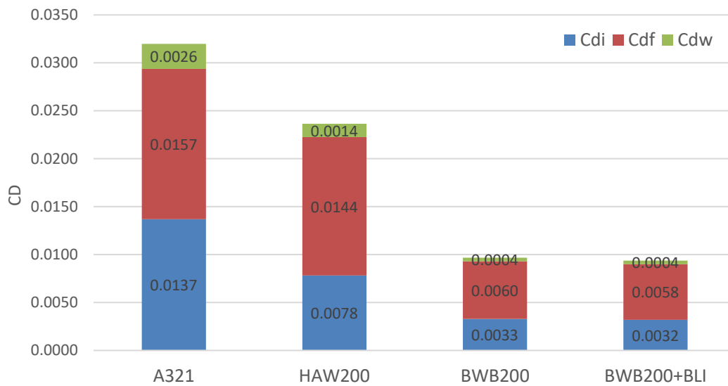
Figure 4-3 Drag build-up for narrow body aircrafts
