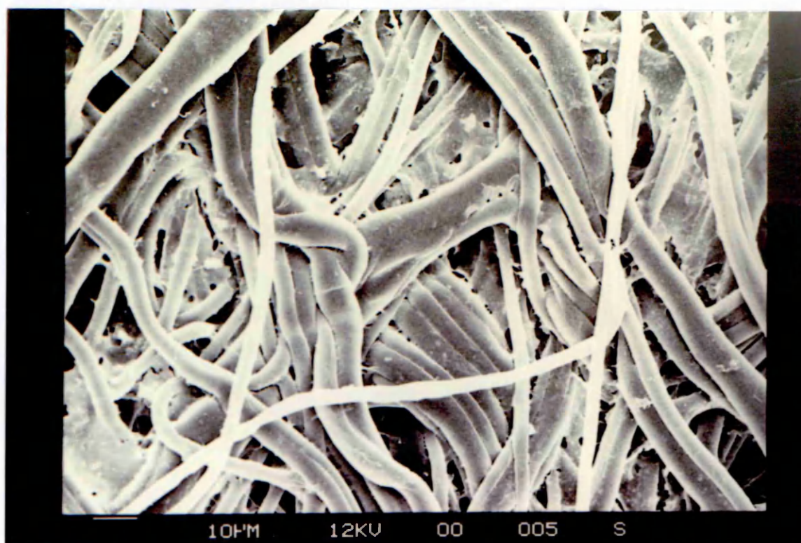
Figure 1 Upper surface SEM view of 1.5 \mu\text{m} non-woven polypropylene membrane material
