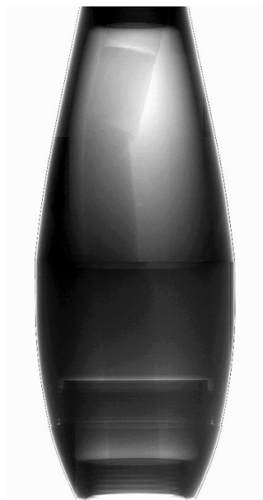
Figure 2.2 Conventional X-ray transmission image of an 81 mm mortar shell with a tube of \text{Al}_2\text{O}_3 through the centre. Image taken at 180 kV, 55 \mu\text{A} with 1415 ms exposure.
