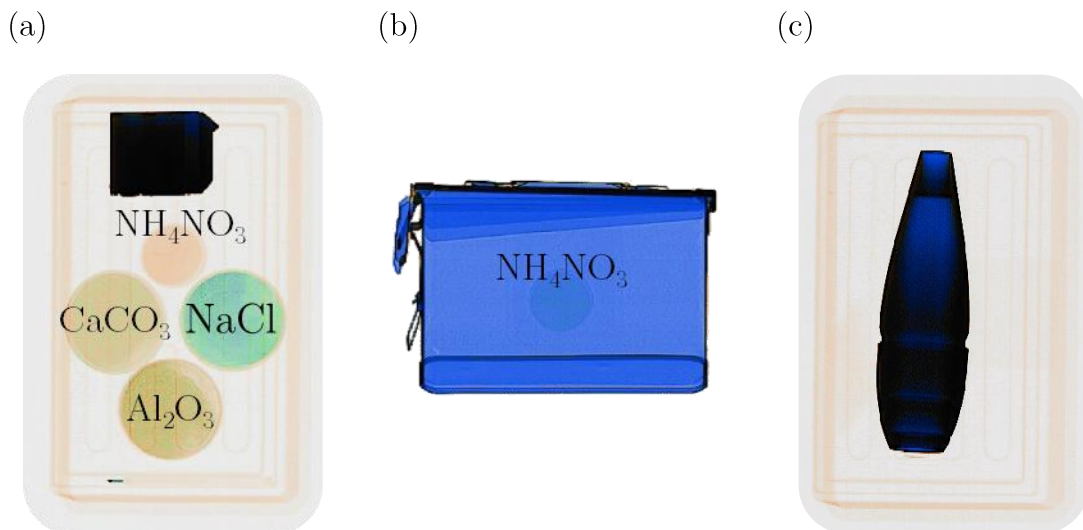
Figure 2.3 Dual-energy X-ray transmission images (a) petri dishes filled with various powder samples and a lead block at the top (b) explosive container with sample of \text{NH}_4\text{NO}_3 in centre and (c) and 81 mm mortar shell composed of iron.
