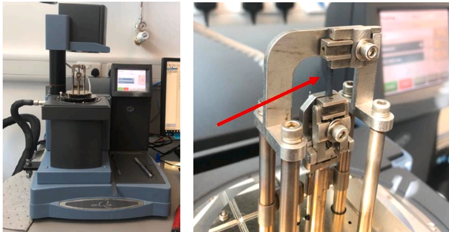
Fig. 5. TA Instruments Q800 DMA (left) and sample in tensile grips (right).
