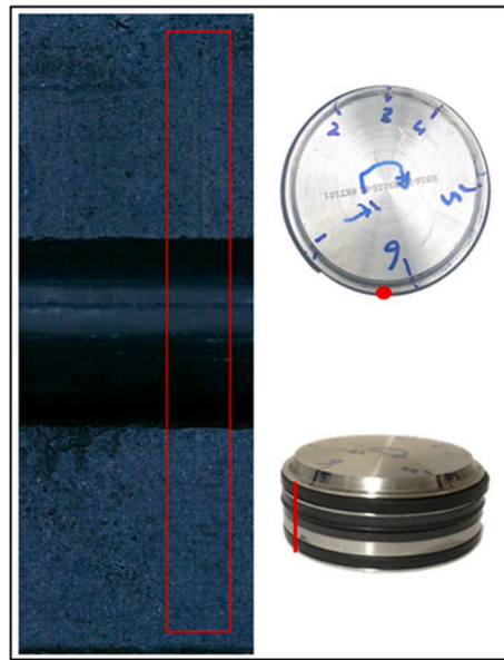
Fig. 11. High- to low-pressure back-up ring wear alignment – section 6.
