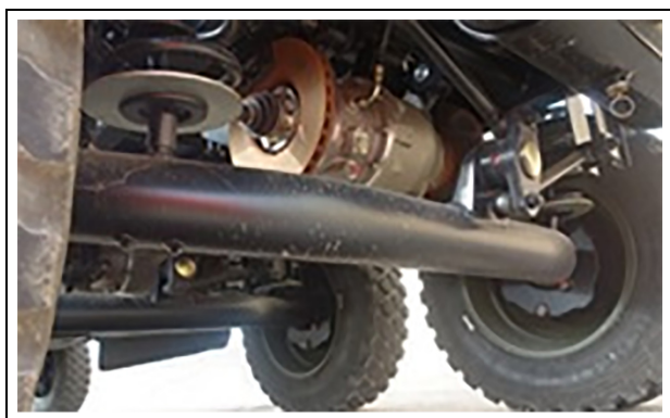
Figure 2. Brake disc installation.
