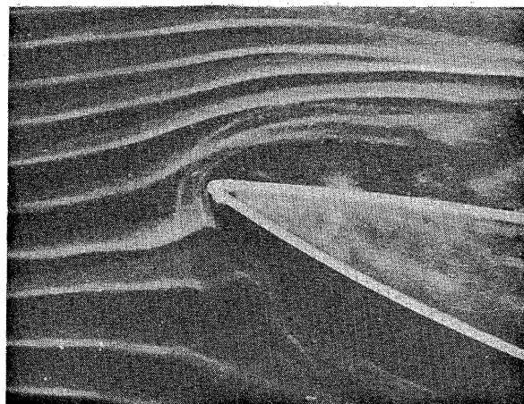
Sharp nose aerofoil at incidence on wall. Incidence \sim 15^\circ
