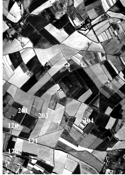
Figure 36. Image of radiance at the sensor (no atmospheric correction) for DAIS channel 76, showing part of the ReSeDA test site with some selected plots indicated. North is up. Radiances range approximately from 0.92 to 1.51 mW/cm 2 sr \mu m (23 to 58 °C).
