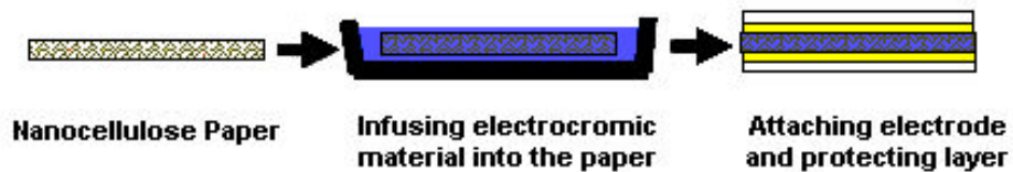
Fig. 18 Fabrication process of the display using nanocellulose
