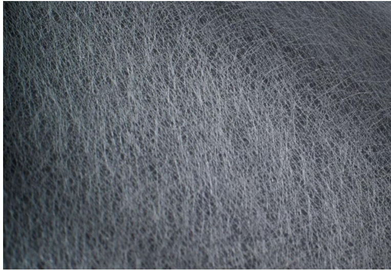
Fig.31 PPS veil interleave material – Technical Fibre Products [280].
