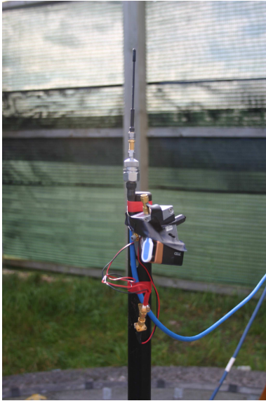
Figure 8. The electrically small monopole connected to a horizontally positioned RF cable.
