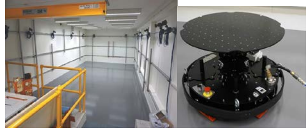
Fig. 5 Left: ORGL epoxy floor. Right: ACROBAT platform (from [4])
