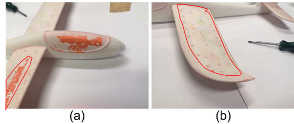
Figure 3. The details of the target aircraft model. The red areas are the damaged area. (a) refers to the right-wing and nose, (b) refers to the left-wing.
