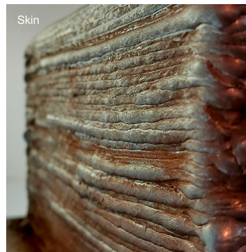
Figure 12. Side view of the demonstrator showing the lower surface roughness of the skin.
