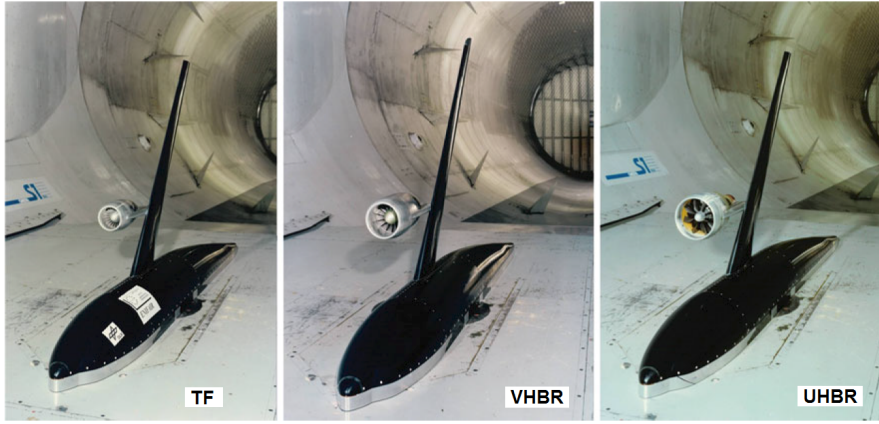
FIGURE 2.16: The comparison of ALVAST airframe 54 with the turbofan simulator (TF), very high by-pass ratio simulator (VHBR) and ultra-high by-pass ratio simulator (UHBR).
