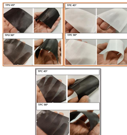
Figure 4-5. The self-cleaning 3D printed textile-like structures with both orientation angle 45 ° - 90 ° for each material.
