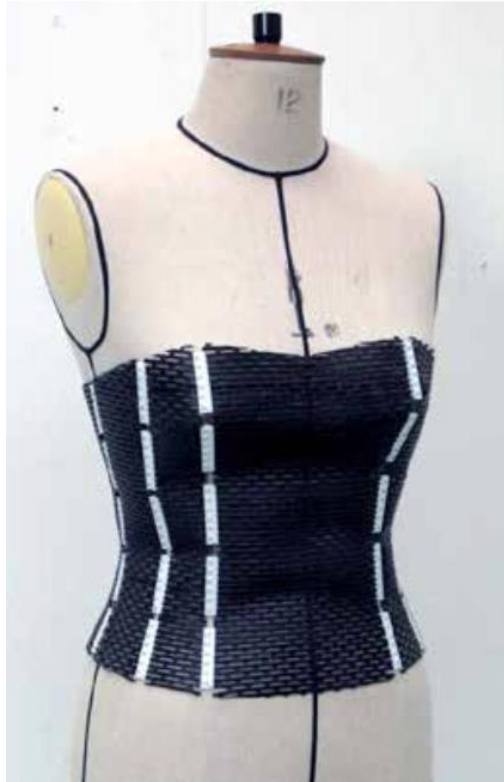
Figure 2-28. The full corset printed with flexible materials [149].
