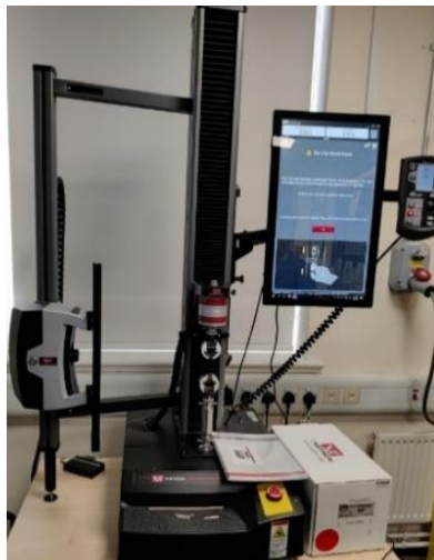
Figure 5-13. An Instron machine for the mechanical strength.
