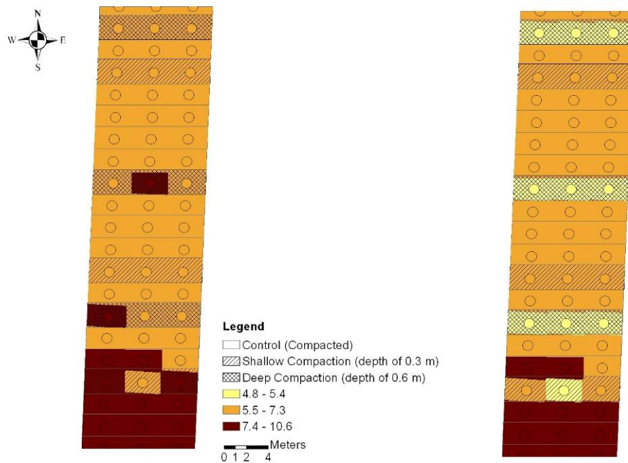
Figure 5.11 Map of EC readings obtained by the Conductometer operated in stationary mode from the trial plot at depth range of 0-0.9 m before (left) and after (right) treatment applying. EC values are displayed in \text{mS.m}^{-1} . Yellow areas (right) represent no compaction above 0.6 m.
