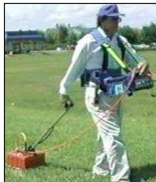
Figure 2.8 Ground penetrating radar (after GeoModel, 2007).
