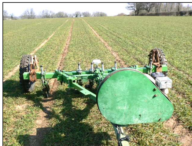
Figure 4.4 Positions of the coulter disc electrodes while running within the tramline.
