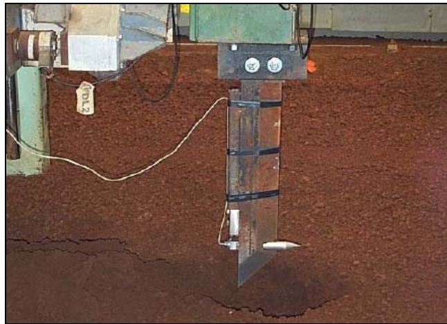
Figure 2.6 Acoustic plow pan detection sensor (Tekeste et al, 2002).
