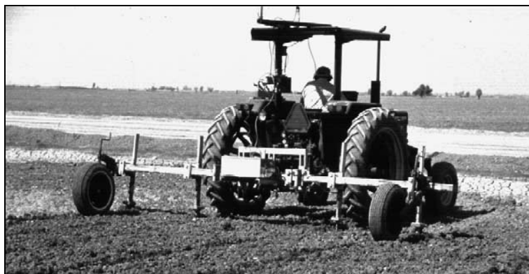
Figure 2.13 Soil electrical resistance equipment developed by Rhoades (1992, 1993).
