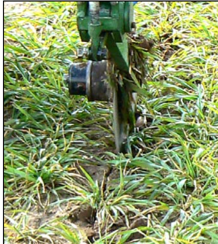
Figure 4.13 Detail view of the disc running in the groove created during the 1 st run.
