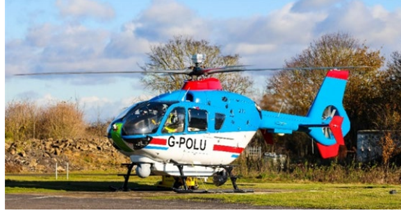
Fig. 5. BladeSense ground runs: H135 helicopter with hub support cap and instrumented blades during a ground run [16].
