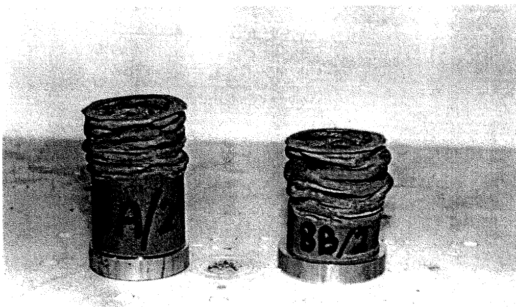
FIGURE 4.14 : Kevlar tubes Batch 8 - Post-test
