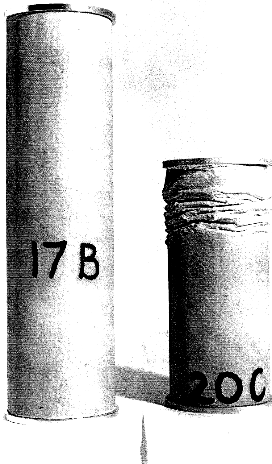
FIGURE 6.15 : Energy Absorbers Intact and Post-crush
