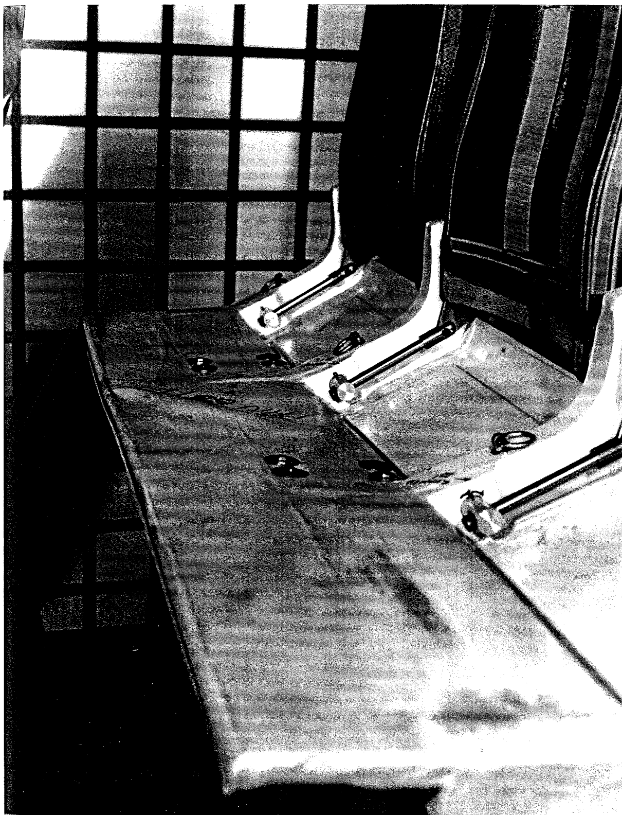
FIGURE 6.8 : Standard Seat during 'Floor Warping'
